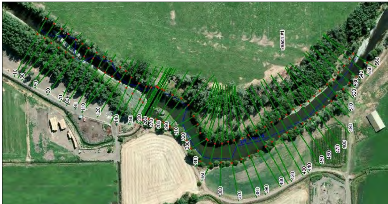
Figure 3-3. Plan view of hydraulic model layout showing cross-section locations.
