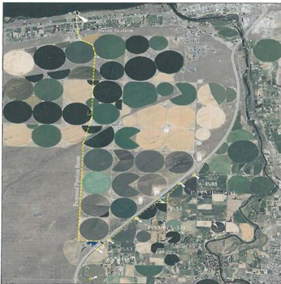
Figure 1: 45 cubic-foot-per-second Columbia River pipeline proposed to be funded and constructed by Westland irrigation District
